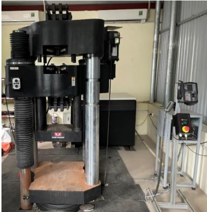
Fig. 5. INSTRON 400HVL 2000 kN testing machine
