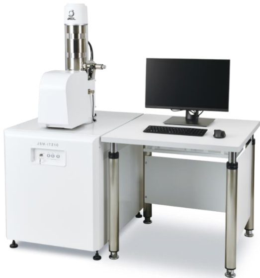
Fig. 6. Scanning Electron Microscope machine for observing the microstructural evolution
