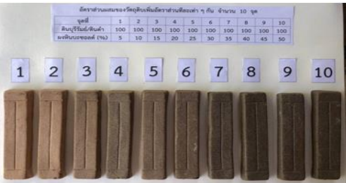
Figure 3: Test Tiles of Ban Kruat Clay and Ball Clay (100 parts) with 5-50% Basalt Stone Powder Addition
